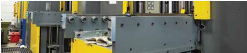
Our facility is home to a multitude of different presses with variable tonnage. KC Seals can manufacture rubber products in diameters ranging all the way from 1/2 an inch to 16 inches, with a maximum height of 10 inches.
