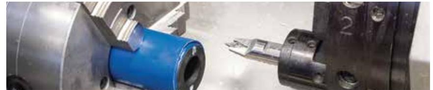
Industry-standard tooling is typically made for the machining of metals. Our CNC lathes are equipped with custom tooling and inserts specifically designed for the manufacturing of rubber. Meaning quality finishes that rival compression molded parts, and tolerances as low as 5 thou.
